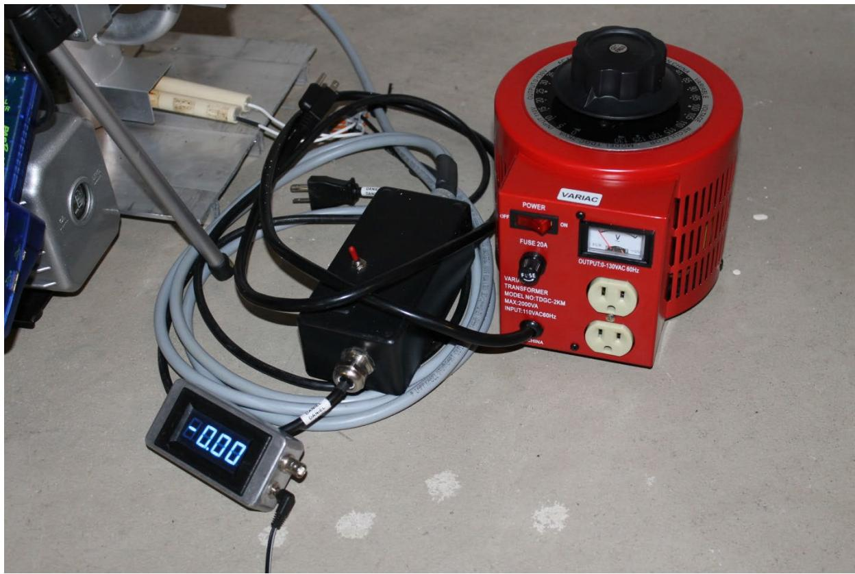
Pictured above is the Variac used for adjusting the primary voltage for the x ray transformer. It is rated for 20 amps.
