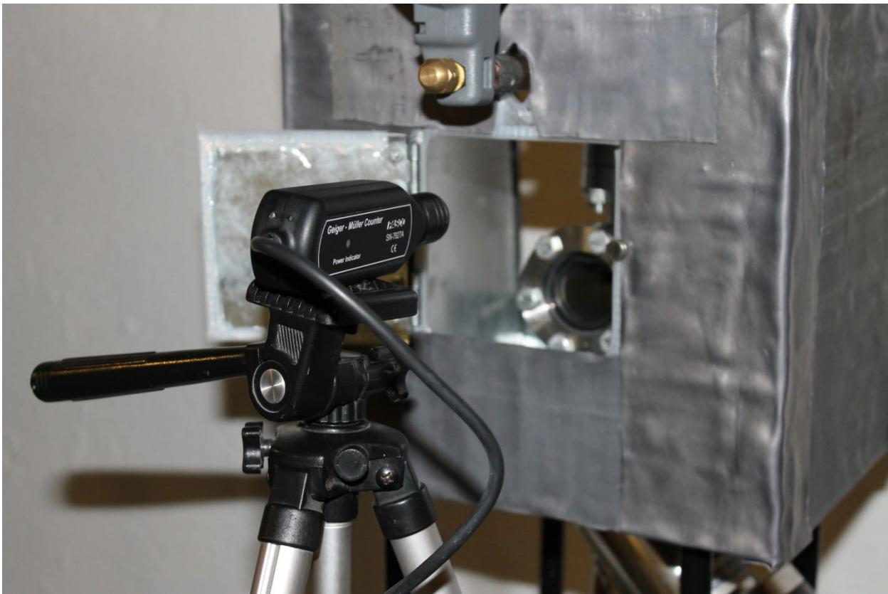
Pictured above is the Geiger-Muller tube on the stand as it was used to record radiation output.
